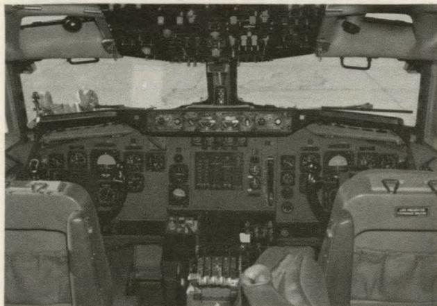
The pilots have an uncluttered, well designed instrument panel and an independent flight director system. The forward aisle panel (knee level) contains the pilot's INS, weather radar, HF and UHF radios.
