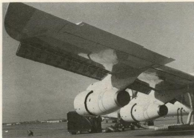
Unlike the 135 models, the E-3A has full leading edge flaps that are extended fully when the inboard flaps reach 6°.
