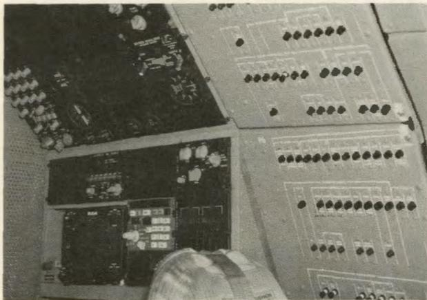
The navigator's station is limited in size and equipment. The navigation computer system (lower right) is essential for mission radar, autopilot control, and overwater flights.
