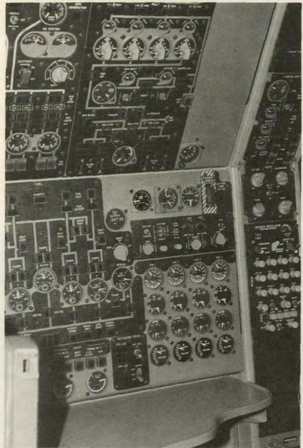
The flight engineer controls and monitors the electrical system as well as the air conditioning, fuel hydraulics, pressurization, and cooling system. The rotodome drive (center bottom) allows the rotodome to rotate at 6 RPM (XMIT) or 1/4 RPM (Idle).
